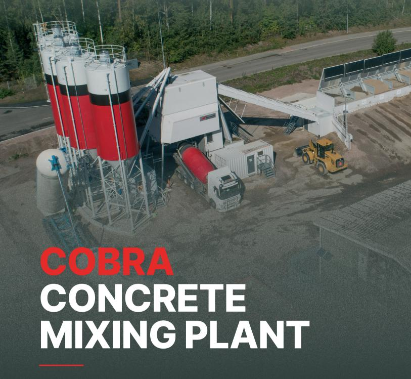
Mobile on-site all season concrete plant for rough conditions. 50 – 160 yd³/h (40 – 120 m³/h).
