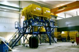
**Color-Mix plant model for top layer concrete** Concrete for wall panel facing or blended blocks and pavers. Changeable aggregate bins. Color pigment dispensing system. Location can be outside or inside the precast factory.
