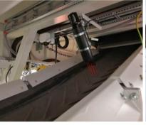
OptiMoist improved aggregate moisture measuring
