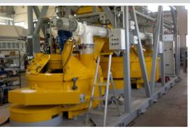
Double mixer set-up Two mixers to increase capacity or for different kind of production.
