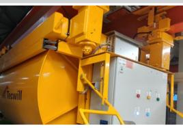
Flying Bucket Concrete Delivery System Wireless ordering system Connection to multiple casting points and machines Duo rails, straight, curved, inclined. Bottom discharge or roll over bucket
